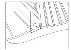
Insert one screw on each side of the top back rail. Use the cocktail stick in the other hole to align with the holes in the top of the back legs.
