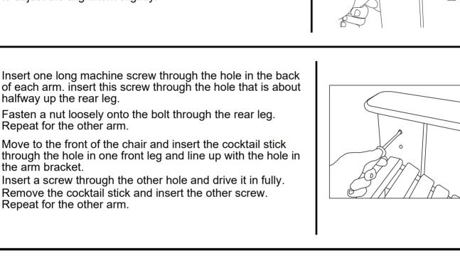
Insert one of the machine screws into each remaining hole (1 on each side), place a nut on the other end and fasten them loosely.
